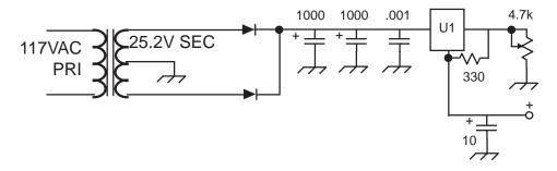
U1 - LM317 voltage regulator. Requires heat sink. All capacitances are in microfarads ( $\mu F$ ), polarized capacitors are electrolytic. Diodes are 1N4001 or equivalent. Resistor is 1/4 watt.
